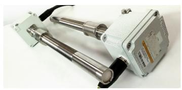
A set of two pipes - probes up to 900 mm long (the length of the probes is specified when ordering). The ends of the pipes are closed with ceramic plugs. The pipes are connected to the emitters of the alarm device by means of a coupling (threaded fitting) with a cylindrical pipe thread of 1" (G1), the pipe material is steel 12X18N10T. A special feature of this version: at the
