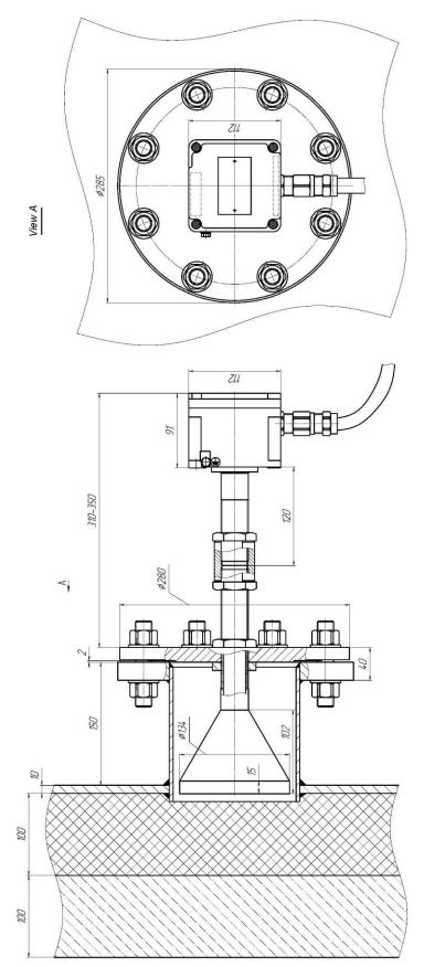
Appendix 3. Drawing of securing TR and RC units with cylindrical emitters on the wall of a concrete bunker
