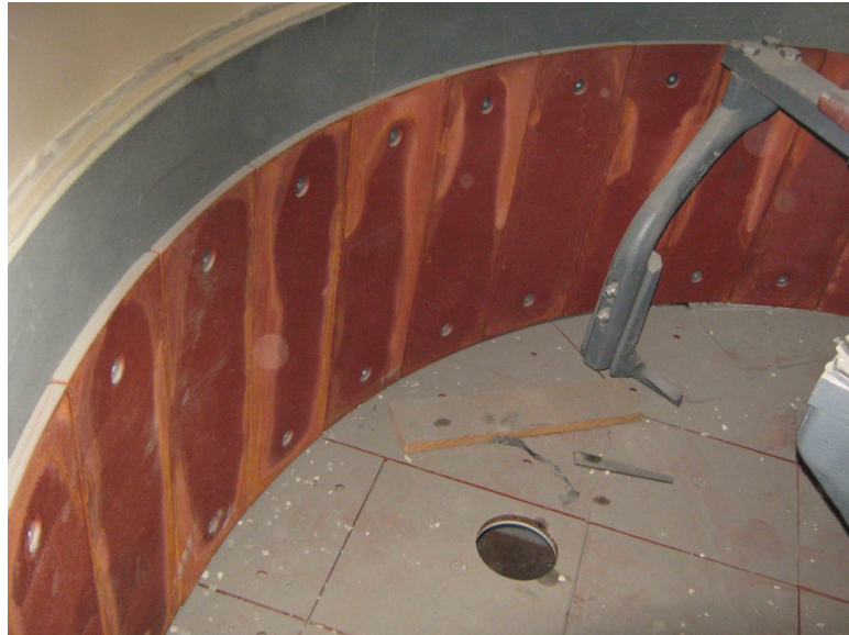
Figure 3. Example of the hole in the concrete mixer floor.
